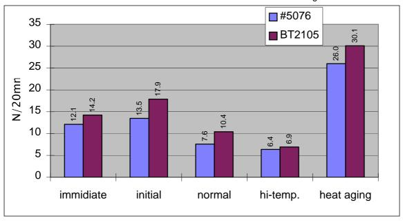
BT2105 V.S. #5076 Adhesion test on "X" head lining.
