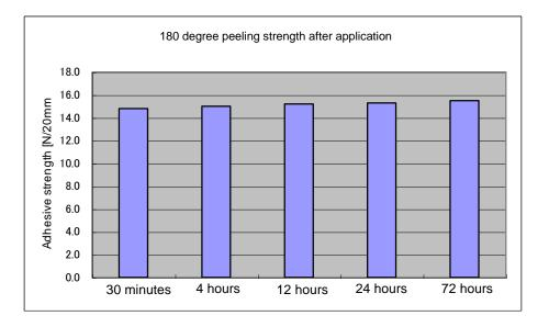
● 180 degree peeling adhesion (2) Long term storage stability
